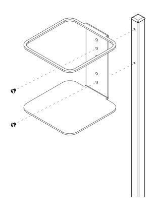
ATTACH THE GALLON HOLDER With the gallon holder holes lined up with the post, fasten the holder to the post using the provided 1/4-20 5/16 in screws and 5/32 in L hex key tool.
